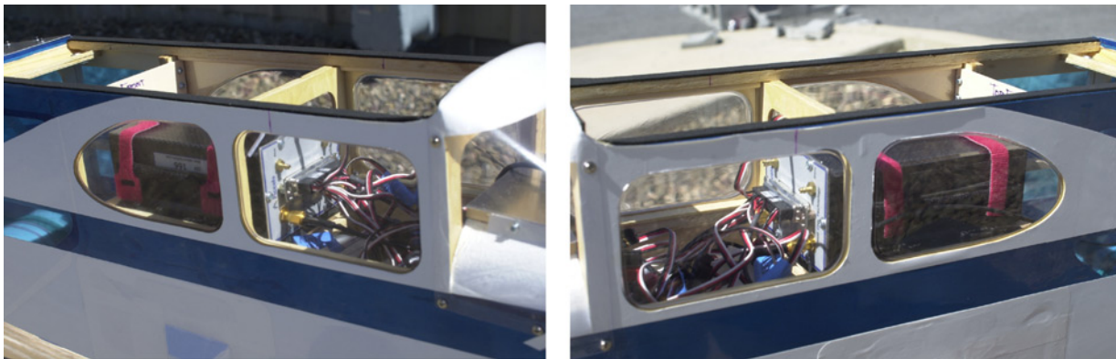
Fig. 7 Left and right views of the autopilot installation.
